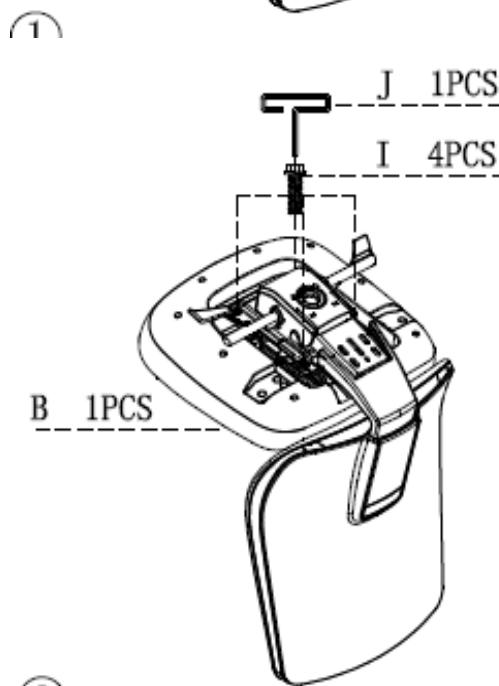
Eng. Assemble Seat B (with seat slider) to the Mechanism C with screw I and wrench J
