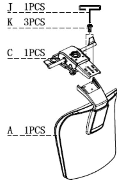
Eng. Assemble the Mechanism C to the Backrest A with 3pcs screws K and wrench J
