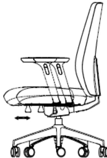
Eng. Press the level ③ and pull the seat to slide forward and backward
