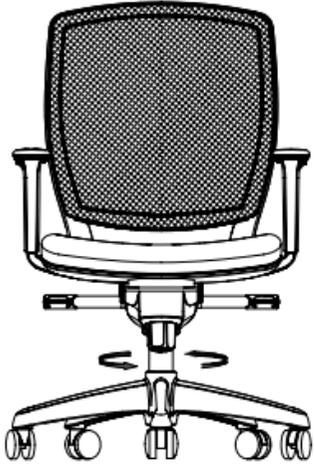
Eng. By turning the big knob you can adjust the tension of the backrest when it is not locked in a fixed position.
