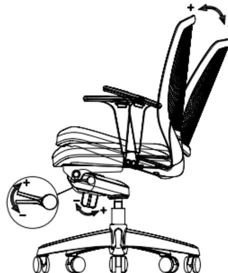
Eng. Push the lever up to unlock the backrest, press it down to lock. It can be locked in 3 positions
